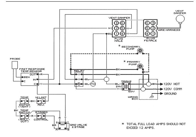
Fig. 22: Primary/Secondary Pumping System Honeywell Zone Valve
